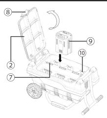
This is a diagnostic charger. The Charger LED Light (7) illuminates in a specified order to show the current battery status. They are as follows:
