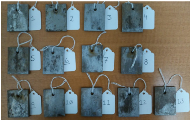
CT-Armor™ 1000 corrosion inhibitor (#3) compared to 12 other corrosion inhibitor tests (720 hours) cleaned.
