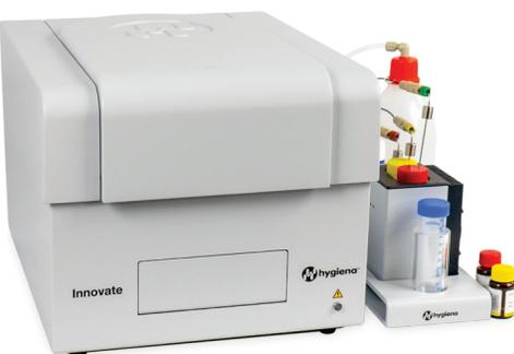
The **Innovate™ System** performs high-throughput screening of products. It rapidly detects adenosine triphosphate (ATP), the energy-releasing molecule found in every living cell. To ensure only microbial ATP is counted, an enzyme breaks down the cell, which isolates microbial ATP.
