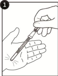
1. Tap Coliform Detection Device on palm of hand 5 times to bring liquid in tube to bottom of tube.
