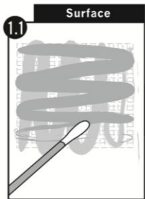
1.1 Surface: Swab 10x10cm area with Enrichment Device.
