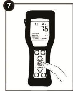
7. If a positive result is obtained for Coliform, presence of E. coli can be verified using E. coli Detection Device. Repeat measurement procedure above using another aliquot sample from same enriched sample.
