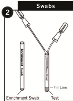
2.1: Swabs: Aseptically transfer 0.1mL (3 drops or to fill line) enriched sample from Enrichment Device to Coliform Detection Device.
