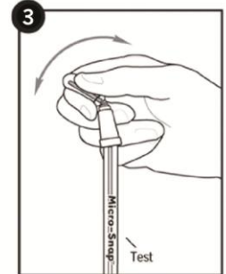
3. Activate Coliform Detection Device by bending bulb forward and backward, breaking Snap-Valve. Squeeze bulb three times to release liquid into tube.
