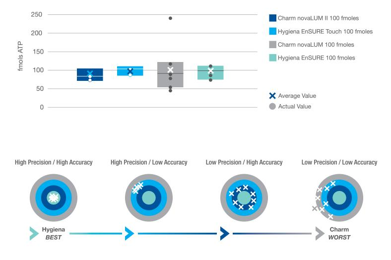
Comparison of accuracy and precision of Hygiena's EnSURE and EnSURE Touch versus Charm's novaLUM and novaLUM II measuring 100 femtomoles with US2020 and PocketSwab Plus ATP swab
