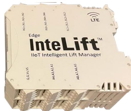
Intelift HPS Well Manager System can be installed with a complete panel or as a stand-alone solution inside an existing Variable Speed Drive or facilities enclosure.
