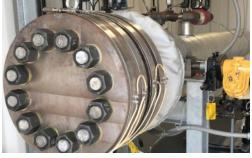
The MLE and cable test pressure vessel is rated for 207 bar (8000 psi) at 343°C (650°F) and is capable of simulating gas decompression events at live well operating temperature utilizing CO<sub>2</sub> and N<sub>2</sub>
