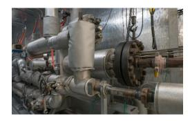
The 260°C (500°F) high-temperature flow loop system tests the ESP performance and reliability at high temperatures, simulating downhole conditions.
