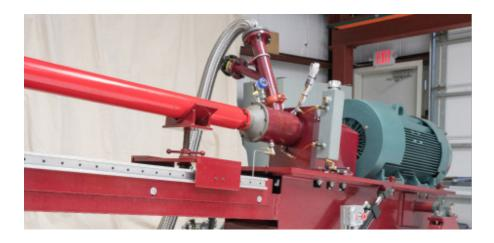
The high-pressure two-phase gas loop simulates and tests ESP components in liquid and gas flow conditions.
