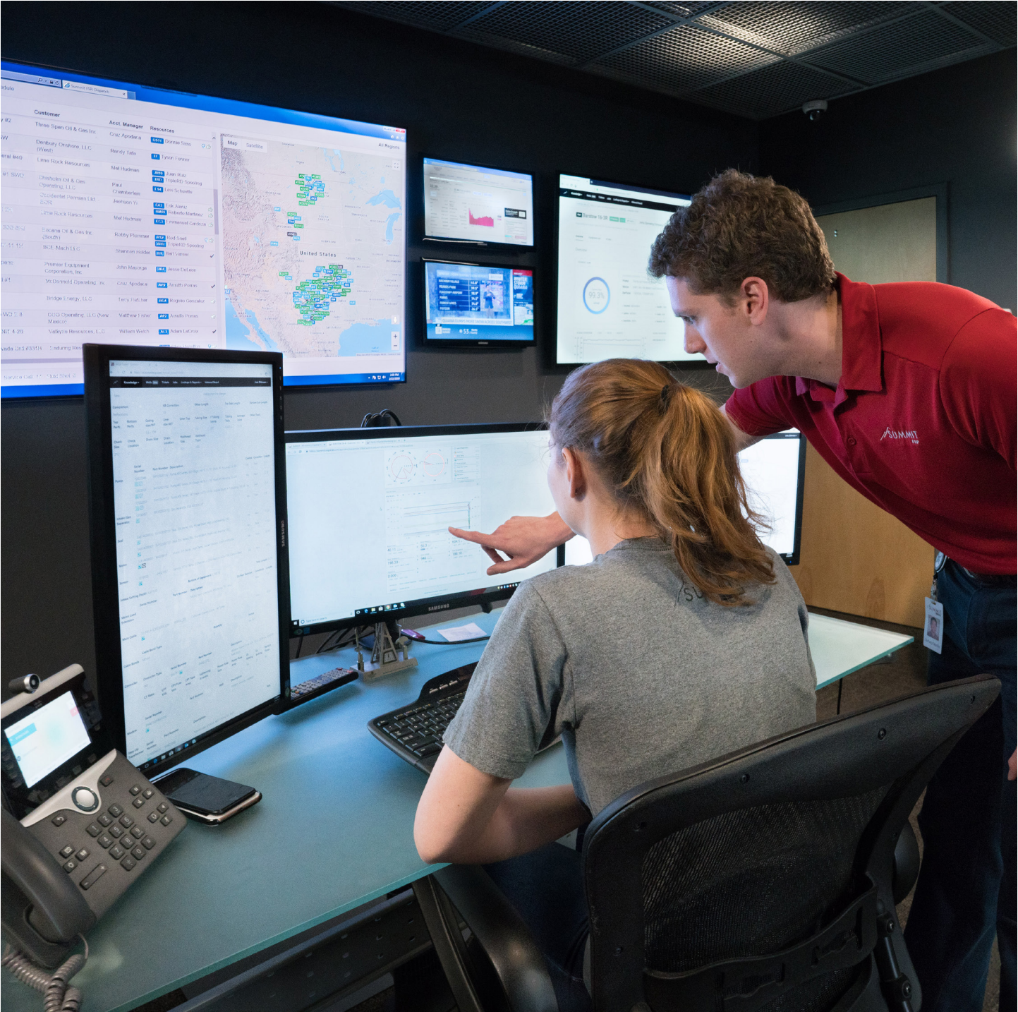
Acquired data from the Triton® gauge is transmitted via modbus protocol or SCADA to a surveillance center through summit ESPs well surveillance and remote control service.
