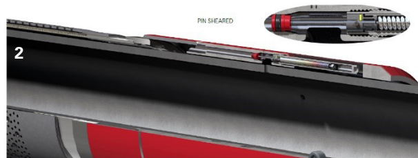
2 Pressure-up to shear pin, plug maintains seal
