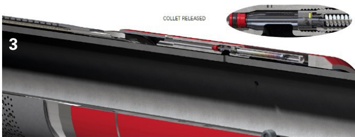
Retaining collet disengages
