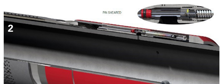
Pressure-up to shear pin, plug maintains seal
