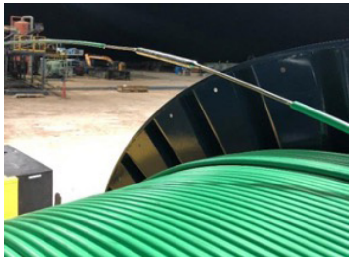
DataSphere Array System is deployed straight from a spool on location. (Source: Halliburton)
