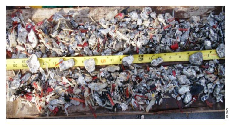
Vali Tech® filter screen recovery of 30.4 lbs aluminum cement, composite and metal recovery during Single-Trip Drillout
