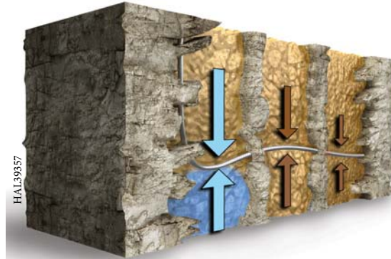
Slotted/Pre-Drilled Liner Standalone Screen Uneven production – early water/gas breakthrough likely, oil production declined
