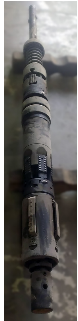
Model 3L™ RBP recovered from well in good condition
