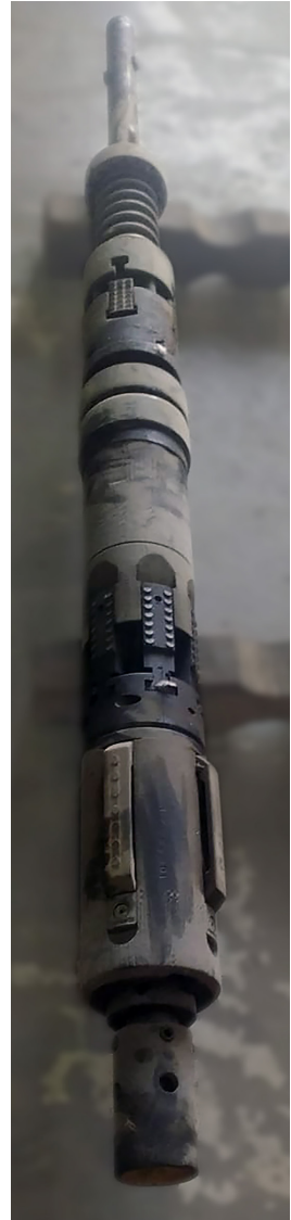
Model 3L™ RBP recovered from well in good condition
