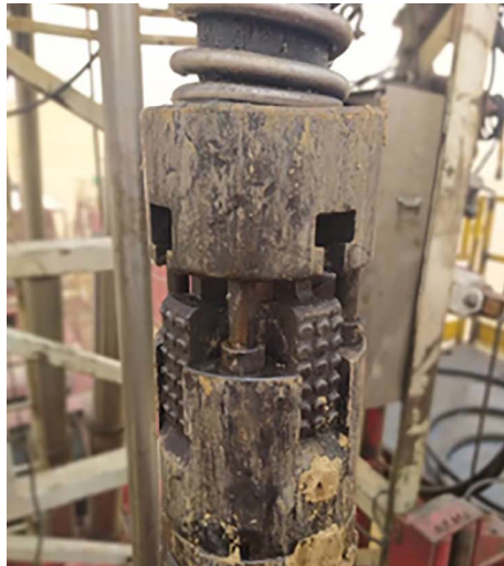
Debris packed off around the Model 3L™ RBP after retrieval.
