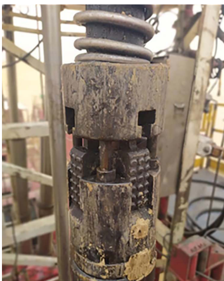
Debris packed off around the Model 3L™ RBP after retrieval.
