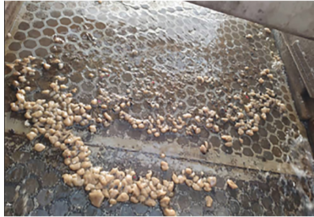
Debris circulated out from above the Model 3L™ RBP prior to retrieval.
