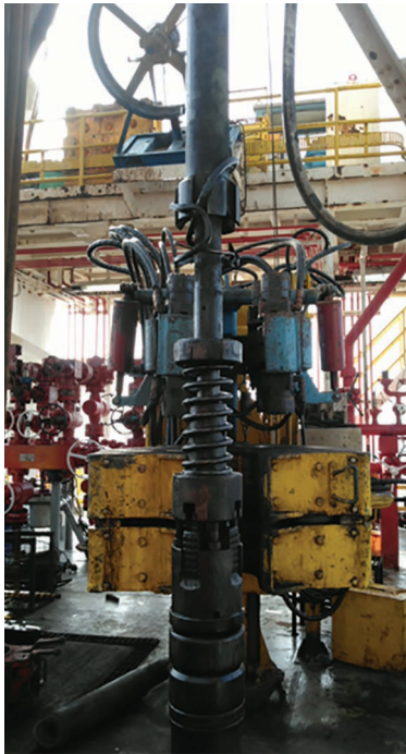
Control line wrapped around the Model 3L™ RBP.
