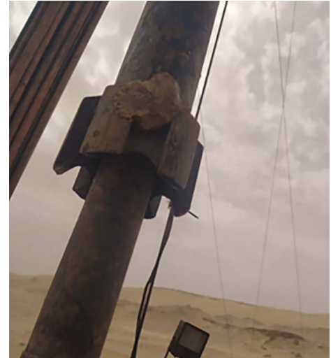
Debris packed off around the Model 3L™ RBP after retrieval.
