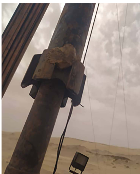
Debris circulated from above the Model 3L™ RBP before retrieval.
