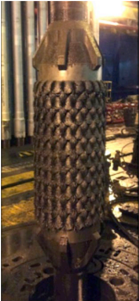
Mag Tech® riser magnet recovers 97.43 lbs of well debris.
