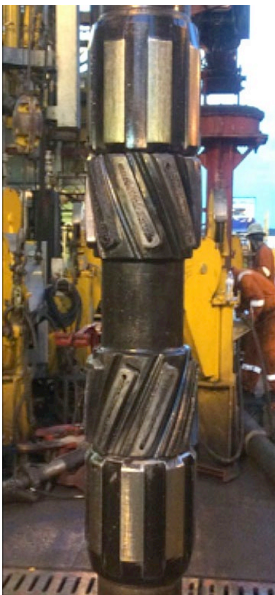
9 7/8-in. Bristle Tech® brush was residue free when pulled out of hole
