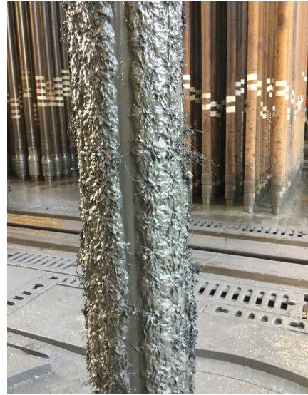
» Swarf collected downhole by PowerMag® casing magnet
