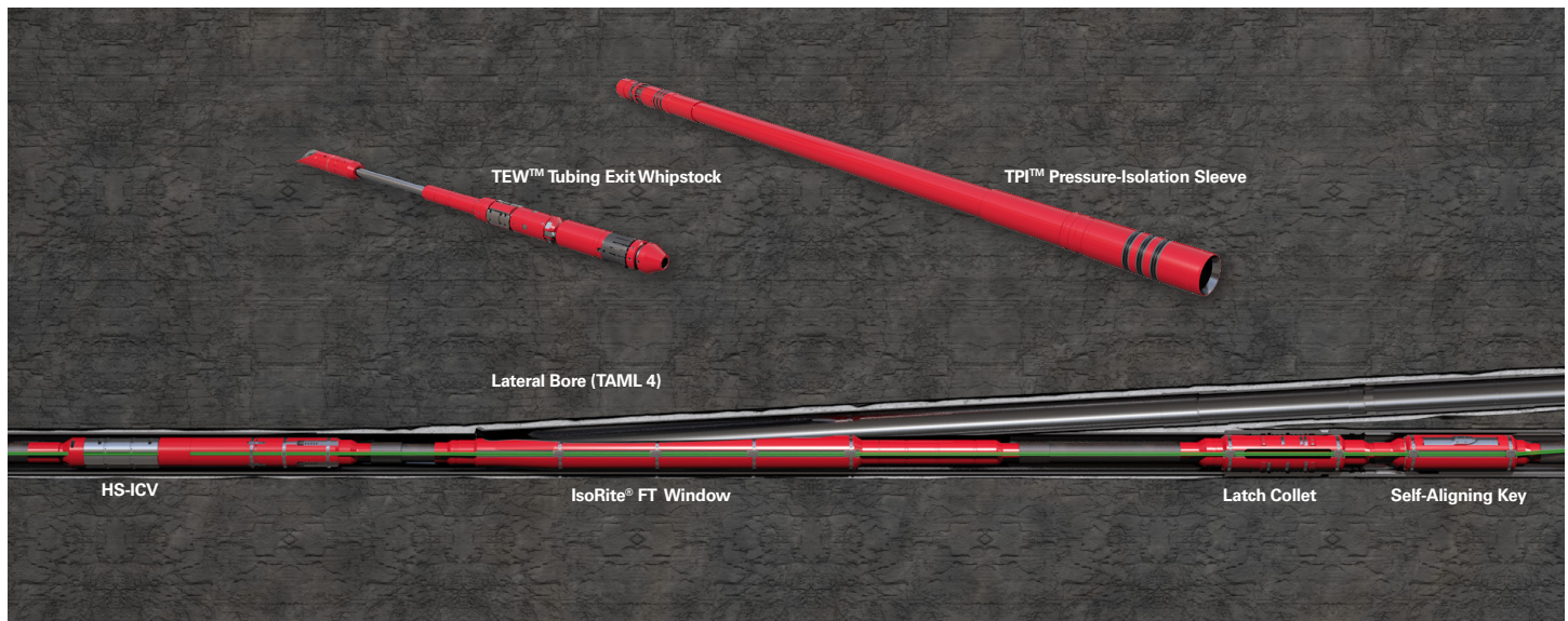
IsoRite® FT completion system in a MillRite® TAML 4 junction
