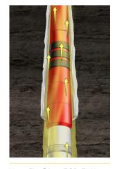
VersaFlex® low ECD ELH system offers approximately twice the annular flow area, thus allowing increased flow rates.
