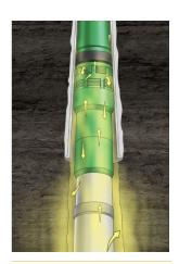
Conventional liner hanger with nominal OD causing a restriction in flow path during well circulation and cement placement, which can damage fragile formations.
