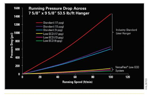
Modeled and confirmed through testing, trip-in-hole speeds and circulation rates are improved up to 90% over industry-standard liner hanger systems.
