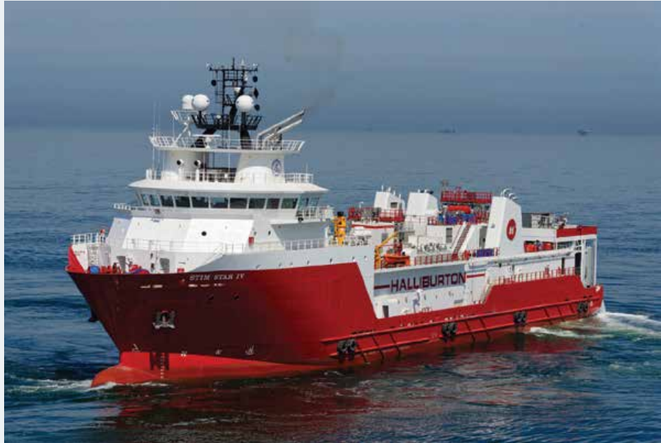
The Stim Star IV has the frac fluid and proppant storage capacity, blending on the fly and high-volume pressure pumping capabilities needed for Lower Tertiary wells in deepwater Gulf of Mexico.
