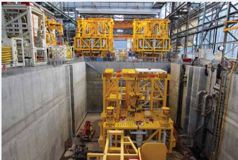
The OneSubsea boosting pumps are rated for 13,000 psi design pressure and differential pressures up to 4,500 psi.
