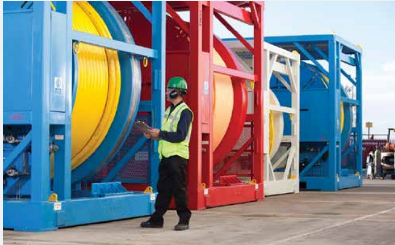
Comprehensive pre-deployment inspection and testing ensured successful installation of the IWOC umbilicals for the Jack/St. Malo project.
