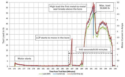
Digital signature plot of a lower crown plug retraction
