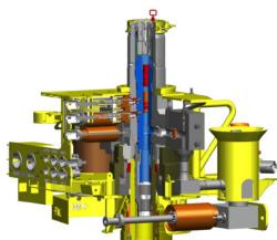
Subsea horizontal wellhead with crown plugs
