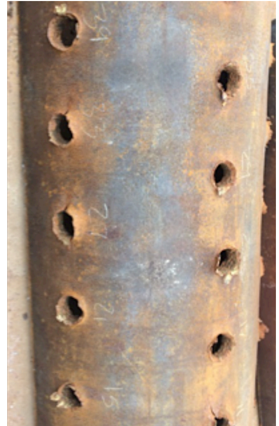
13 \frac{3}{8} -in. casing after perforation.
