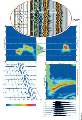
This is an example of a semblance diagnostic plot of the waveform data from the eight waveforms. In the circle is a section of a log showing monopole P-wave slowness and semblance quality, monopole-refracted shear-wave slowness and semblance quality, X-X dipole slowness and semblance quality, and Y-Y dipole slowness and semblance quality.
