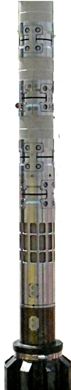
The Xaminer Sonic Imager excites the Stoneley mode in the borehole over a wide frequency range (300 Hz – 5 kHz).
