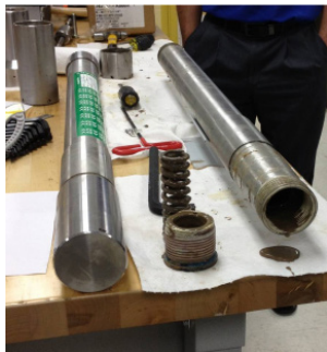
Disassembled CoreVault tubes after lab analysis is complete.
