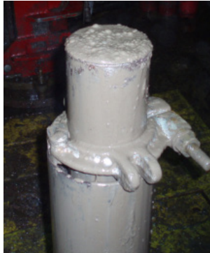
At surface, gas bubbles out of a conventional core.
