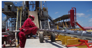
Large-volume coring tool being prepped for run.
