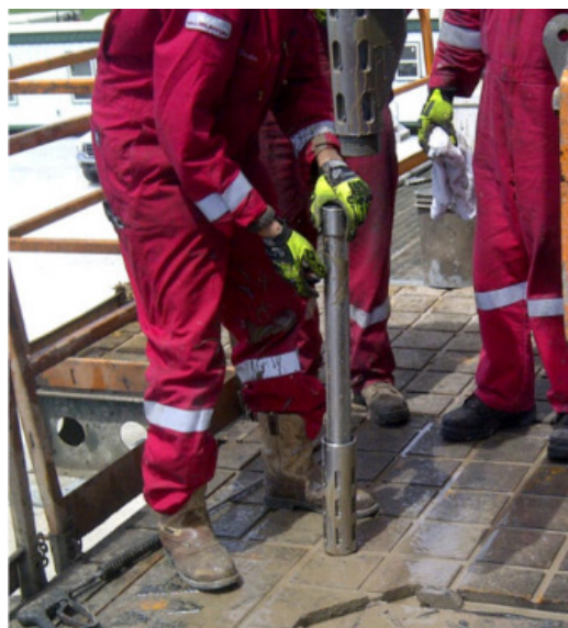
Specialists remove the CoreVault® tool from the wellbore.
