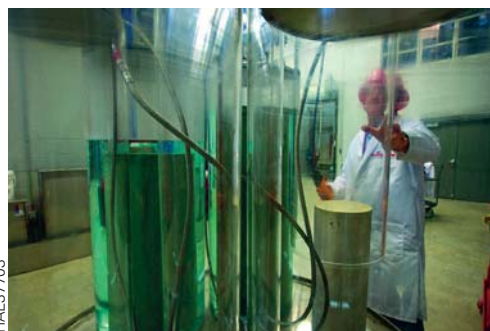
Cores taken from the field and analog rocks are prepared and analyzed before testing in the flow vessels.
