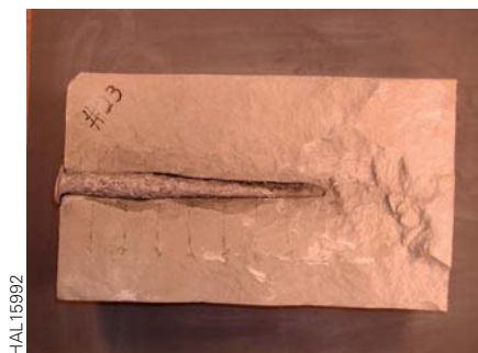
Berea test shot balanced with effective stress at 3,000 psi and dynamic volume at 1,430 cc.
