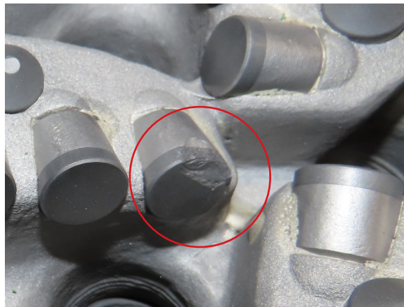
Significant wear flat and thumbnail crack (tangential overload) that has mechanically propagated and partially failed.
