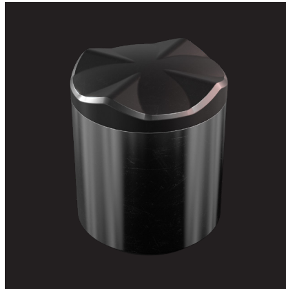
Razor shaped cutters are designed with higher contact stress along the cutter rock interface to fail rock more effectively.
