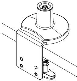
**1.** Attach base clamp to table top. Tighten clamp to hold in place.
