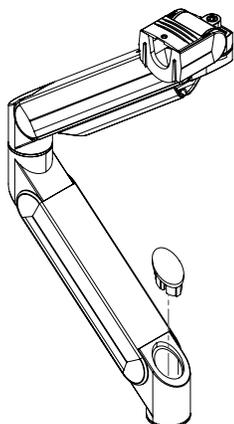
3. Insert the rubber cap into the opening in the monitor arm.
