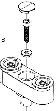
**b.** Remove the plastic cap and take out the M8x35mm screw and M8 washer located beneath it.
