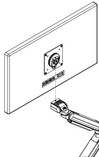
5. Gently press down the monitor mounting plate into the opening at the top of the monitor arm. Note the locking plate at the top of the monitor arm may be blocking the opening and will need to be slid into the unlock position to expose the opening.
