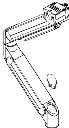
**4.** Insert the rubber caps into the openings in both monitor arms.
