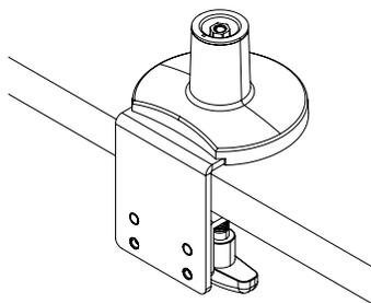
1. Attach base clamp to table top. Tighten clamp to hold in place.
