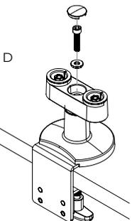
**d.** Secure the branch adapter to the base clamp using the previously removed M8x35mm screw and M8 washer. Use the provided tools to tighten the screw in place. Reattach the plastic cap in the same position it was removed from.
