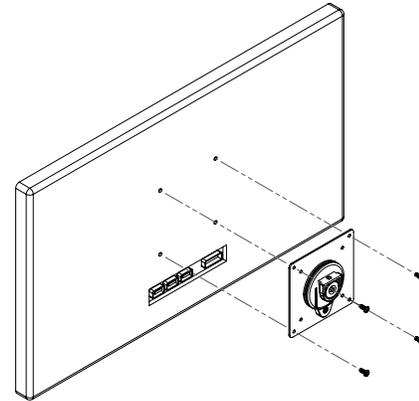
4. Attach the monitor mounting plate to the back of the computer monitor using four provided M4x10mm screws.
