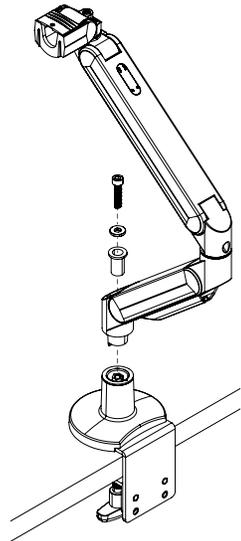
2. Insert the monitor arm into the base clamp. Slip the black bushing, M8 washer and M8x35mm screw into the opening in the monitor arm. Tighten the M8 screw in place using the provided tools.
