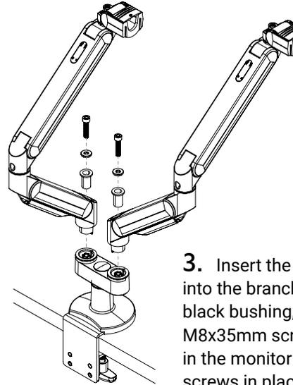
**3.** Insert the dual monitor arms into the branch adapter. Slip the black bushing, M8 washers and M8x35mm screws into the openings in the monitor arms. Tighten the M8 screws in place using the provided tools.
