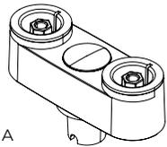
**2.** Assemble the branch adapter to the base clamp.
