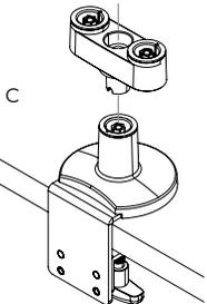
**c.** Insert branch adapter into base clamp.
