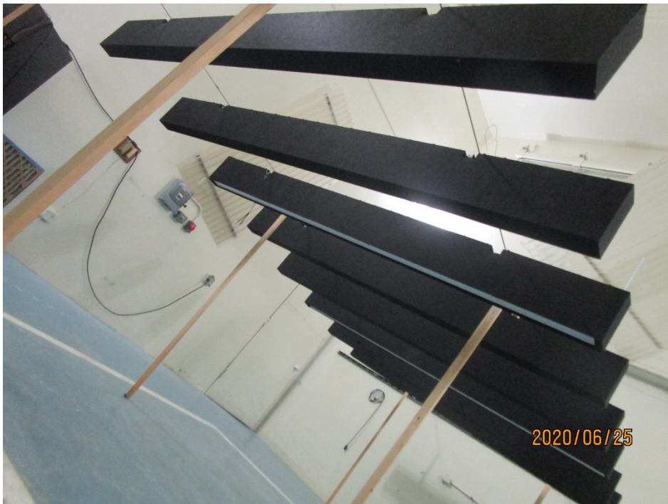
Figure 2 – Underside of specimen, position of baffles with light fixtures
