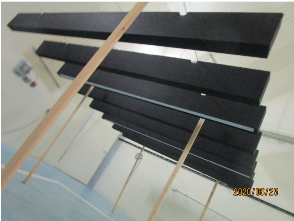
Figure 2 – Underside of specimen, location of baffles with light fixtures
