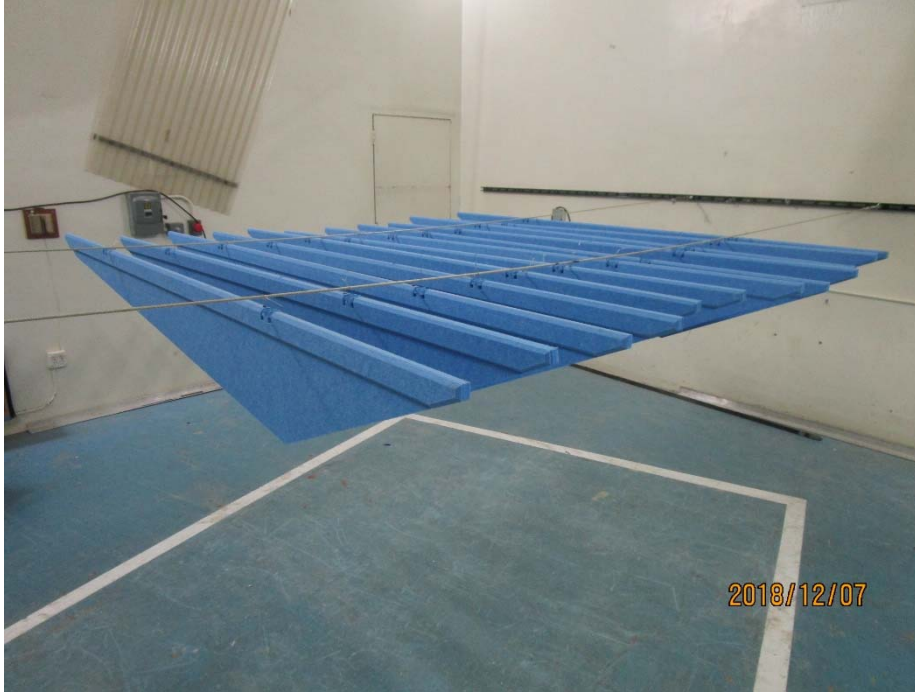
Figure 1 - Specimen mounted in test chamber, type 1 baffle mounted closest to south test chamber wall
