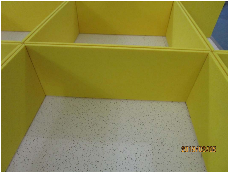
Figure 2 – Detail of specimen materials, typical Switchblade joints
