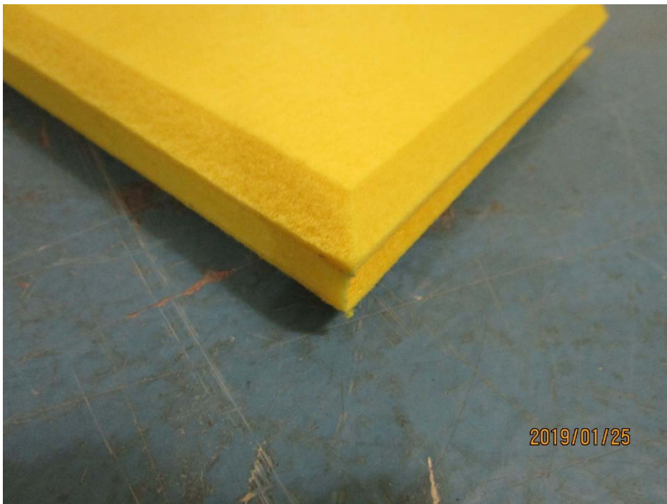
Figure 4 – Detail of Switchblade material and chamfered edges
