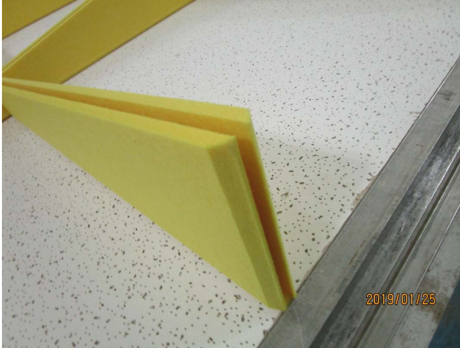
Figure 3 – Detail of Switchblade material and chamfered edges
