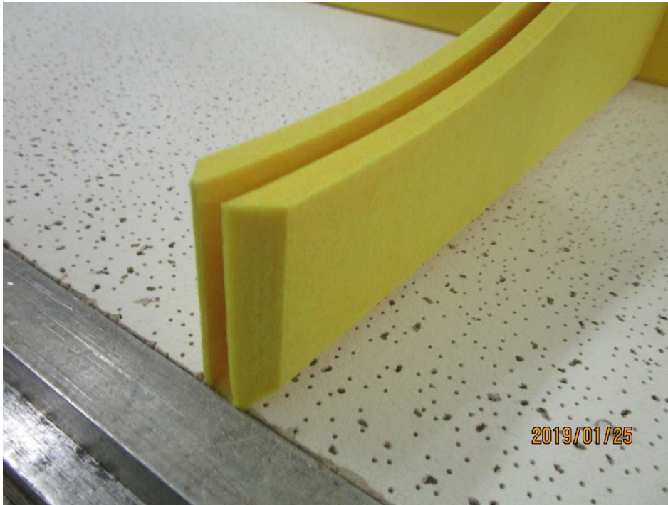
Figure 3 – Detail of Switchblade material and chamfered edges
