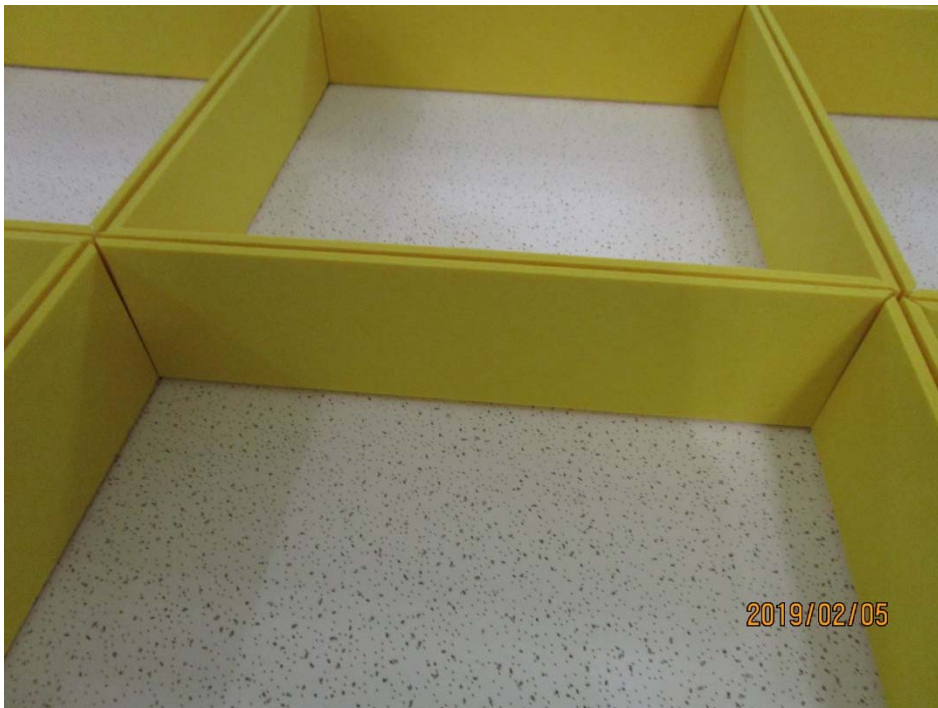
Figure 2 – Detail of specimen materials, typical Switchblade joints
