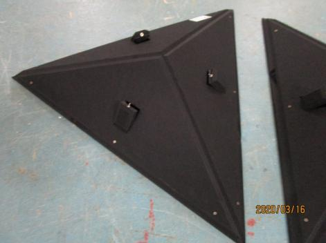
Figure 3 – Top face of individual fixture
