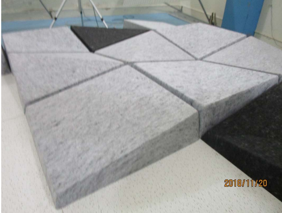
Figure 3 – Layer 2 partially installed over Layer 1
