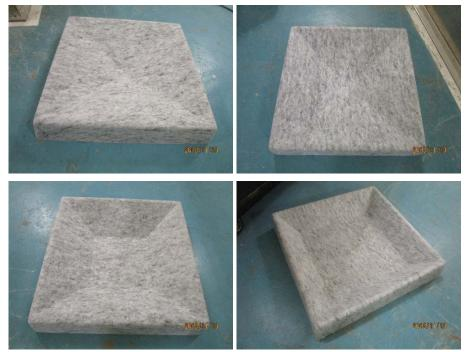
Figure 2 – Port tile types A (upper left), B (upper right), C (lower left), and D (lower right)
