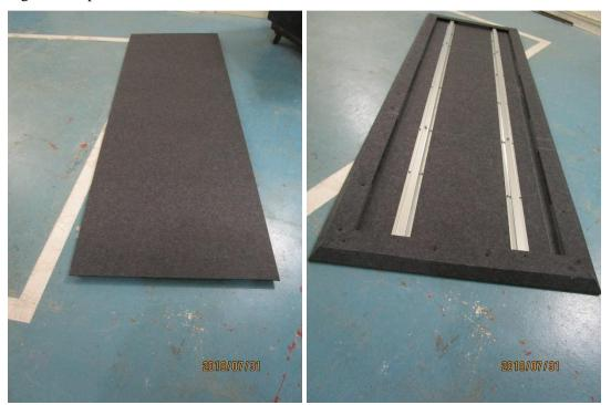
Figure 2 – Individual baffle, sides facing sound field (left) and horizontal test surface (right)
