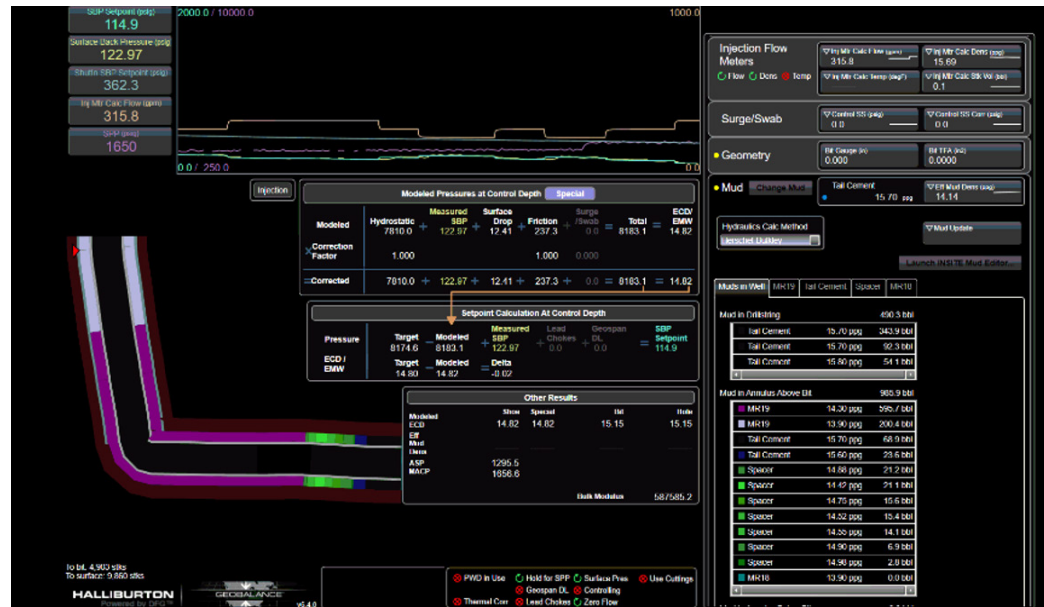
Graphic shows hydraulic model accurately tracked actual mud density throughout the annulus. This automated data input into the software and eliminated all manual entry usually necessary during each stage of cementing.
