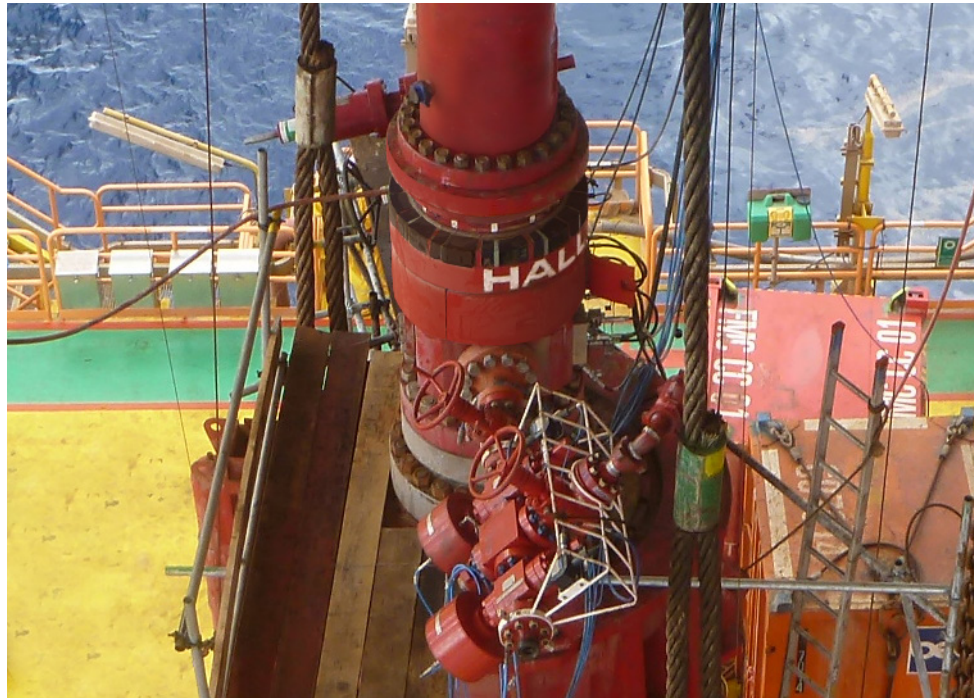
The Marine Sentry RCD 3000™ rotating control device and the GeoBalance® MPD system were key components of an engineered solution enabling an operator to safely drill a reentry well in the Gulf of Mexico.
