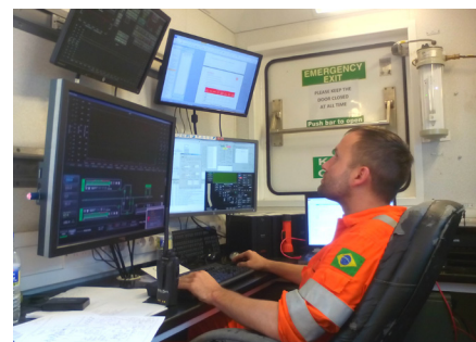
Monitoring real-time information, the Halliburton global GeoBalance® team ensures the MPD system is maintaining constant bottomhole pressure.
