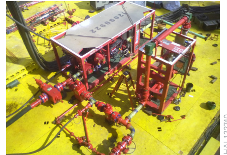
The Halliburton MPD choke and Coriolis meter installed on the rig.
