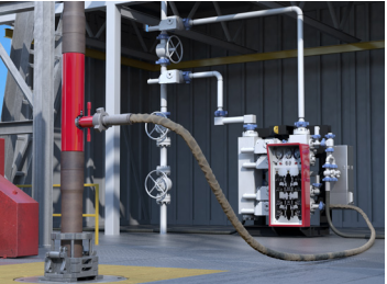
This view shows the process of adding a new stand. A new stand has been installed on the top drive, but before the side port connection has been removed.
