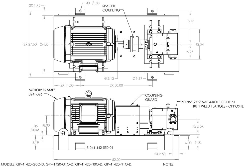
MODELS: GP-41420-G0O-D, GP-41420-G1O-D, GP-41420-N0O-D, GP-41420-N1O-D, GP-41420-K0O-D, GP-41420-K1O-D, GB-41420-K0O-D, GB-41420-K1O-D, GB-41420-N1O-D, GB-41420-R0O-D, GB-41420-R1O-D
