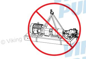
**NOTE: NEVER** lift the unit with slings unsecured under the base. The slings can slide, allowing the unit to tip and/or fall. Improper lifts can result in personal injury and/or damage to the unit.
