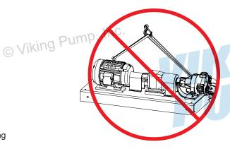
NOTE: NEVER lift the unit with slings connected to the component lifting features. The lifting features are designed for the individual component and are not rated to lift the entire unit, Improper lifts can result in personal injury and/or damage to the unit.
