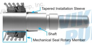
**NOTE:** Coat rotor shaft, tapered installation sleeve and inner diameter of mechanical seal with P-80<sup>®</sup> or equivalent before assembly.
