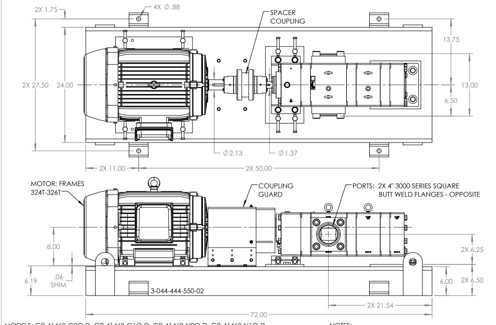
MODELS: GP-41460-G0O-D. GP-41460-G1O-D. GP-41460-N0O-D. GP-41460-N1O-D. GP-41460-K0O-D, GP-41460-K1O-D, GB-41460-K0O-D, GB-41460-K1O-D, GB-41460-N0O-D, GB-41460-N1O-D, GB-41460-R0O-D, GB-41460-R1O-D
