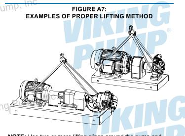
**NOTE:** Use two or more lifting slings around the pump and the motor when the base does not have lifting features. Make sure the slings are secure and the load is balanced before attempting to lift.
