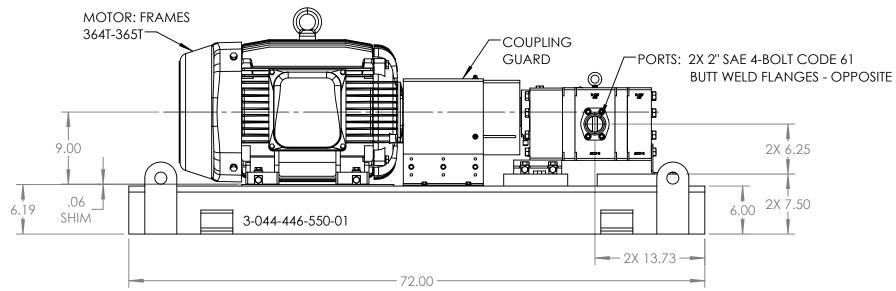
MODELS: GP-41430-G0O-D, GP-41430-G1O-D, GP-41430-N0O-D, GP-41430-N1O-D, GP-41430-K0O-D, GP-41430-K1O-D, GB-41430-N0O-D, GB-41430-N1O-D, GB-41430-R1O-D
