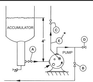
Schematic of Piping and Valves for a Liquid Ammonia Recirculating Pump in a Refrigeration System
