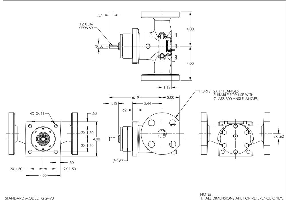
THIS DRAWING IS THE PROPERTY OF VIKING PUMP, INC. AND IS PROPRIETARY IN GENERAL AND DETAIL. IT SHALL NOT BE COPIED OR ITS CONTENTS REVEALED TO OUTSIDE PARTIES WITHOUT THE WRITTEN CONSENT OF VIKING PUMP, INC. DIMENSIONS ARE IN DWG. NO. 05/09/2017 VIKING PUMP, INC. A Unit of IDEX Corporation Cedar Falls, IA 50613 U.S.A. SHEET 1 OF 1 REV. B.O STATE Released INCHES DRAWN 05/09/2017 sjakel PROJECT: GV-1474 05/09/2017 05/09/2017 WAS: CHECKED BAM
