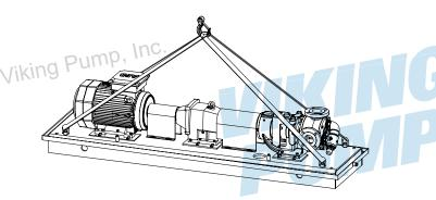
**NOTE:** Units should be lifted by the base lifting features using two or more lifting slings.
