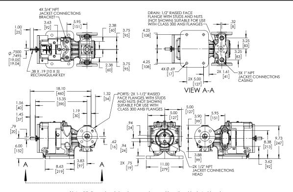
Note: All dimensional drawings are shown with optional jacketed head. These dimensions are average and not for construction purposes. Certified prints on request.
