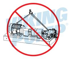
NOTE: NEVER lift the unit with slings connected to the component lifting features. The lifting features are designed for the individual component and are not rated to lift the entire unit. Improper lifts can result in personal injury and/or damage to the unit.
